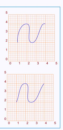
Perhaps the influence of the invisible endpoints is better illustrated, if we draw both the \pscurve and \psecurve together. The next picture does this for the two sets of points in the above example, where the portion of the \pscurve not drawn by \psecurve is shown in a lighter color.
