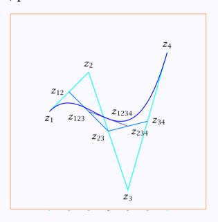
How about the other points of the curve? Well, the process we've described above is repeated with the new control points  $z_1, z_{12}, z_{123}, z_{1234}$  and  $z_{1234}, z_{234}, z_{34}, z_4$  to get another point and so on *ad infinitum*. This process converges rather quickly and the scaffolding is finally removed.<sup>1</sup>
