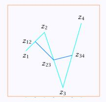
These three points are again joined by straight lines and then the midpoints of the two line segments are found. Let them be  $z_{123}$  and  $z_{234}$ . These two points are joined by a straight line and the mid point of this line segment is found.
