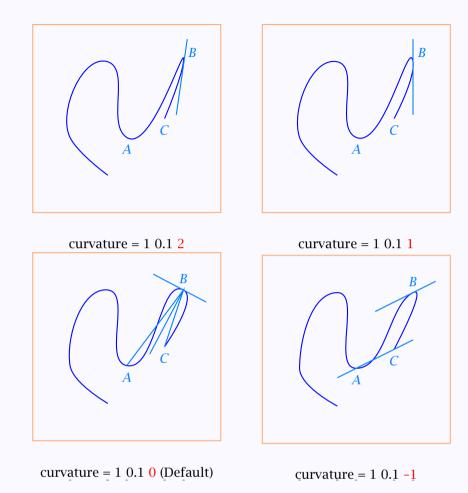
Note how decreasing the third number rotates the tangent at *B* counterclockwise.
