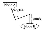
**Incangle** is also a good way to join nodes by a right angle, with just two line segments, as in this example:
